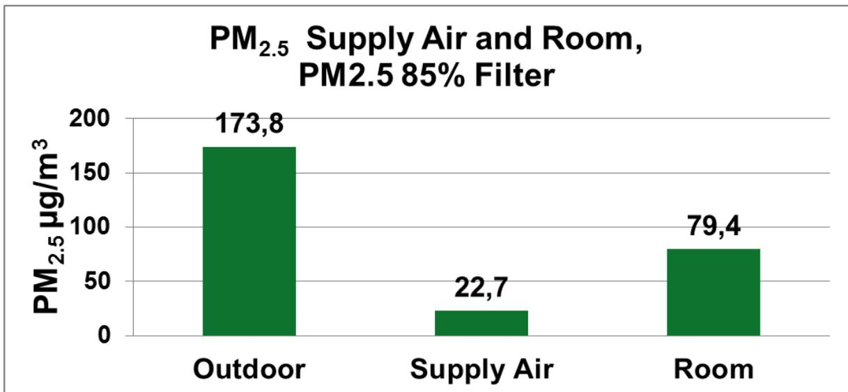
Figure 7: Shanghai Office during working hours, day with poor outdoor air quality
