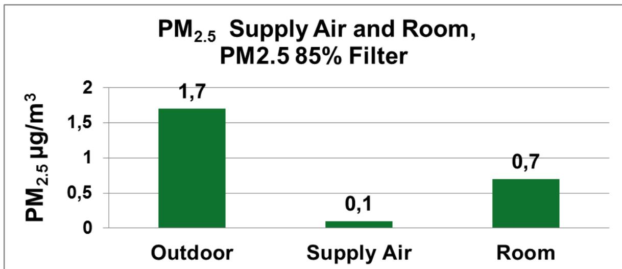
Figure 5: Air quality in office with PM<sub>2.5</sub> 85% filters in Gothenburg
