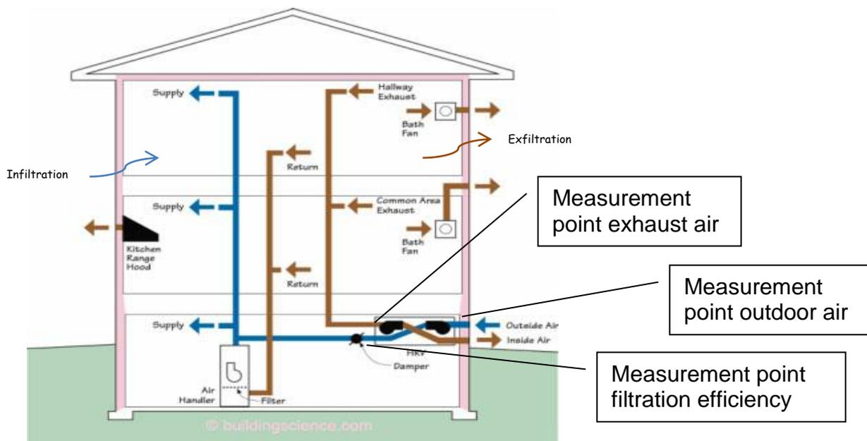
Figure 2 – Description of general ventilation system [11]
