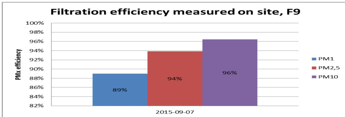
Figure 5 Office building in Gothenburg, PM<sub>x</sub> removal efficiency for F9 filters
