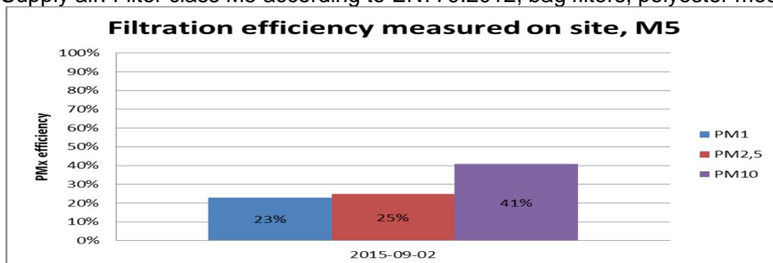
Figure 3: Office building in Gothenburg,  $PM_x$  removal efficiency for M5 filters
