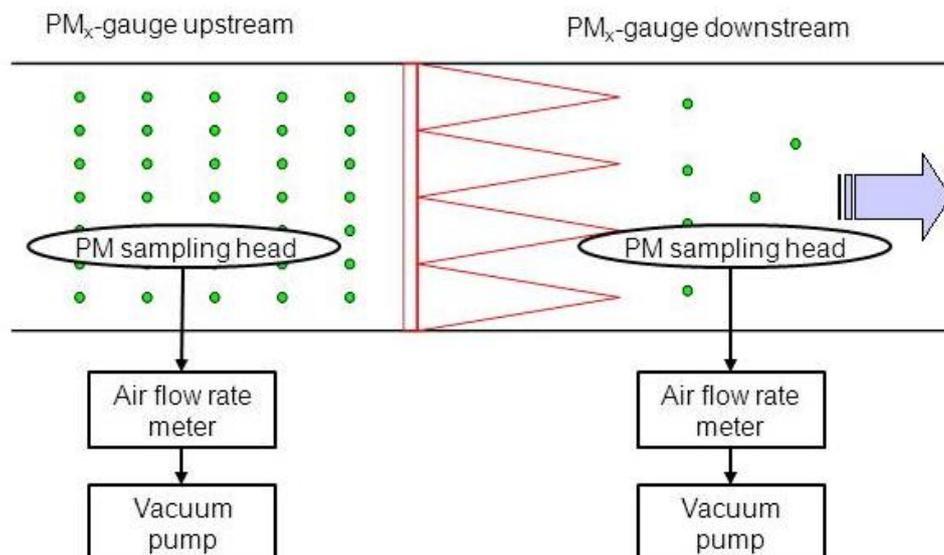
Figure 5, In situ measurement setup
