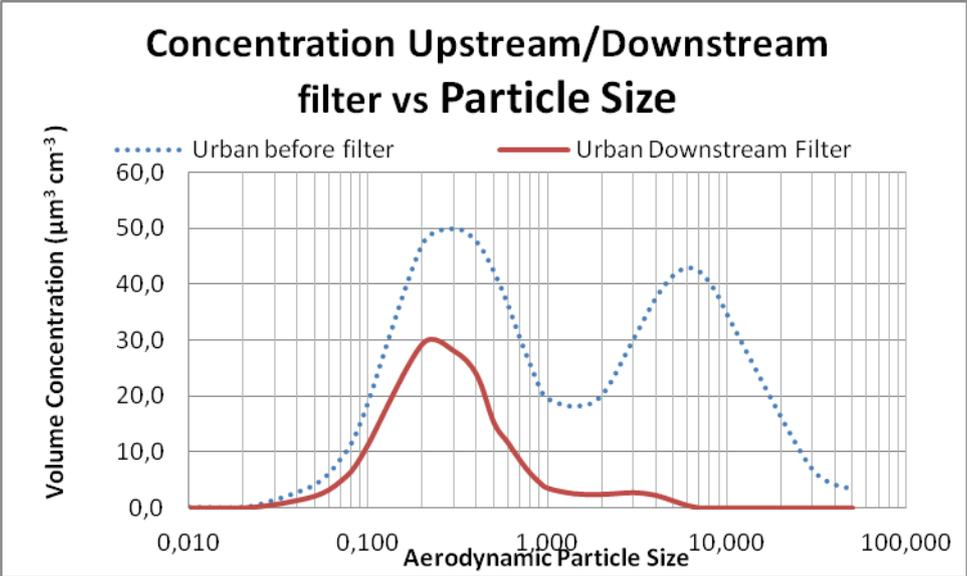
Figure 3, Particle distribution upstream and downstream a filter of filter class F7
