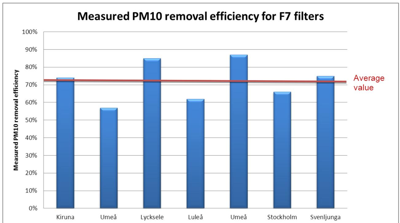
Figure 7, PM10 removal efficiency measured in different places of Sweden
