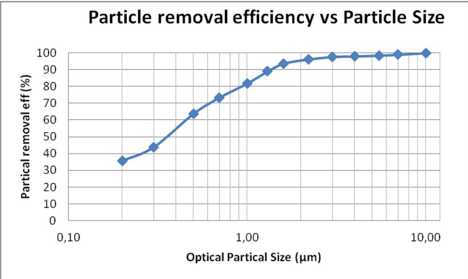
Figure 1, Filtration efficiency vs. particle size for clean filter of filter class F7
